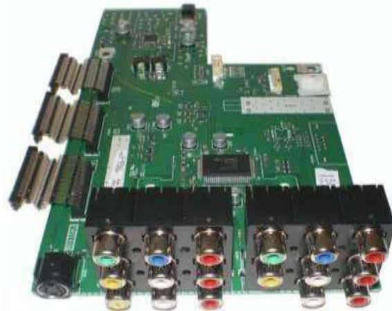
LCD TV jack pack/Input atau signal board
