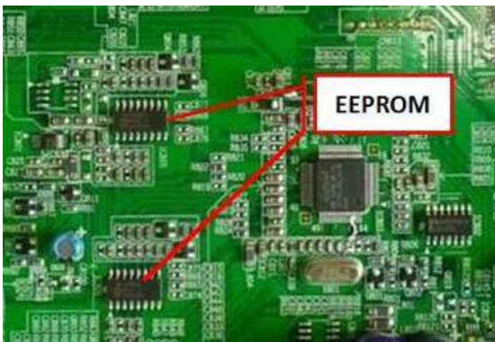
EEPROMS on LCD TV mainboard
