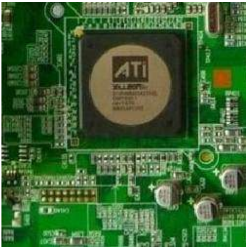
VPU on LCD TV main board
